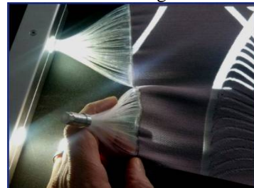
4- Connection of fibers to light sources with lenses
